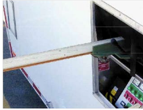
Figure 2.12 Recovered lead painted siding is fed into the planer on one side of the trailer
