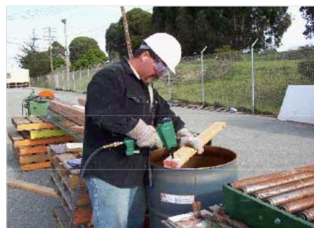
Figure 2.8 Pneumatic de-nail station with the "Nail Kicker" ( www.nailkicker.com )
