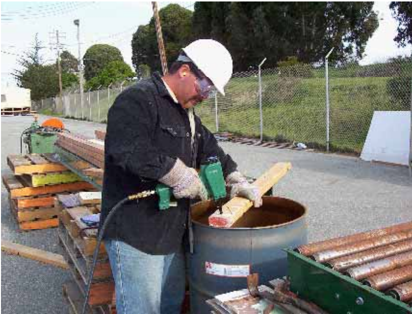
Figure 2.8 Pneumatic de-nail station with the “Nail Kicker” ( www.nailkicker.com )
